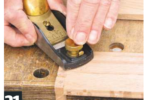
21 Once glue has dried, trim protruding dovetails flush with finely set block plane
